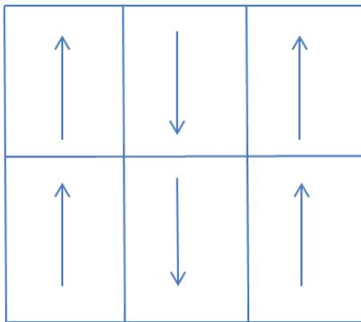
6. Lay the rolls to provide as few seams as possible with economical use of materials. All rolls being installed on a given day must be unrolled the day before and allowed to relax overnight.
