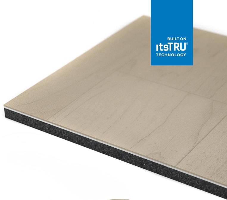
Baller Motivate Class I is designed specifically for courts and multipurpose rooms and features a 2mm vinyl surface layer factory fusion bonded using itsTRU<sup>®</sup> technology to a 5mm Class I VCR base layer to create a Class I sports floor. The Baller wood visuals are designed to replicate traditional wood court visuals and can be combined with the Baller solid colors to create court accents and borders.
