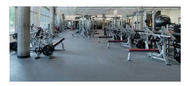
floor features a 2.5mm VCR surface fusion bonded to a 12mm VCR base layer using itsTRUTM technology. The result is a floor designed to withstand extreme weight impacts while minimizing bar bounce. Using Performance Beast Plus with Performance Rally creates the ideal fitness floor solution without transitions.
